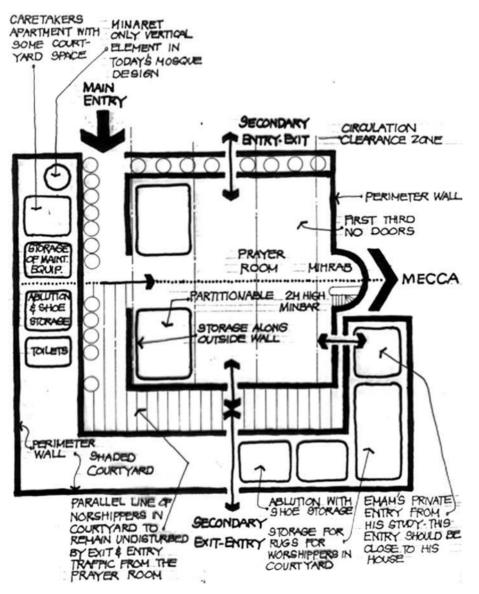
Figure 4.3 Generic plan for an urban mosque showing various typical interrelated functions and their placement
